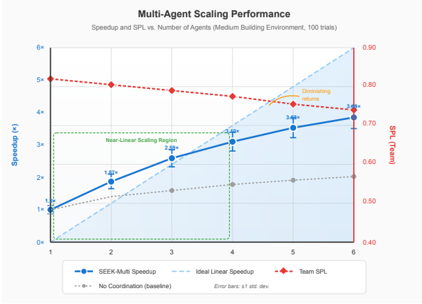
Fig. 3: Search efficiency vs. number of agents. SEEK-Multi achieves near-linear speedup up to 4 agents, with diminishing returns beyond due to coordination overhead. Error bars show standard deviation over 100 trials.
